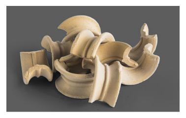
A low-pressure-drop random packing design, such as the FLEXISADDLE<sup>®</sup> LPD<sup>®</sup> media from Knight Material Technologies, shown above, can limit nesting and reduce pressure drop by 20% or more compared to standard RTO saddle media.
